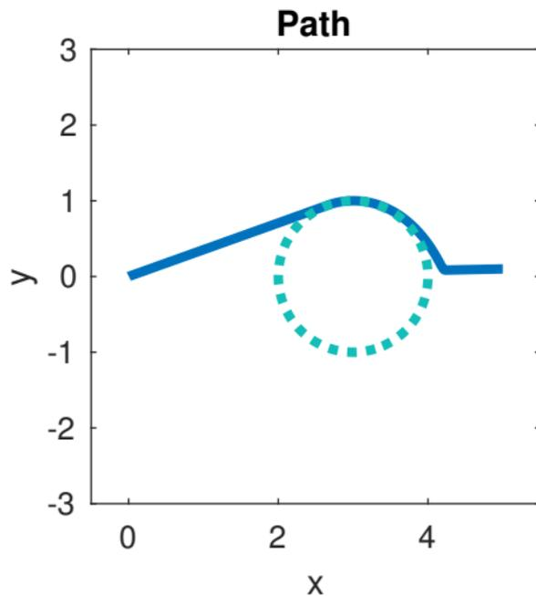
Figure: Trajectory with single obstacle
