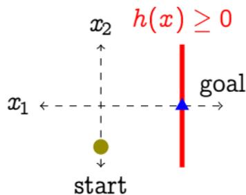
$$L_f h + L_g h u + \lambda h \geq 0 \iff a^\top (Ax + Bu) + \lambda (a^\top x + b) \geq 0$$
